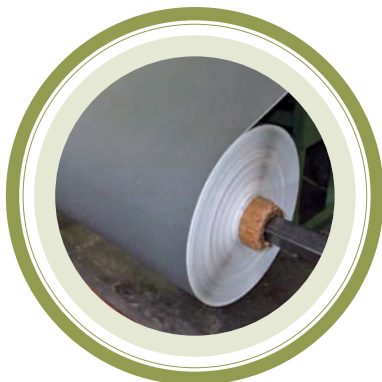
08 Washed, neutralized and cured Savutec® vulcanized fibre
